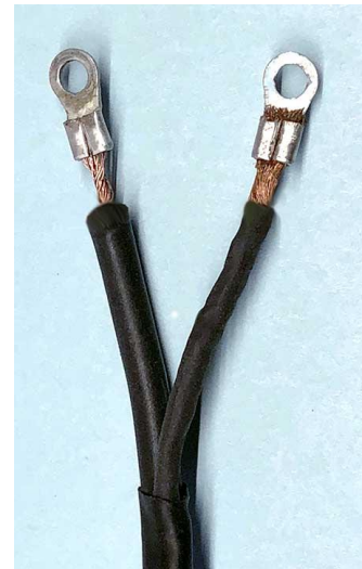
Figure 6: Coax pigtail ends.
